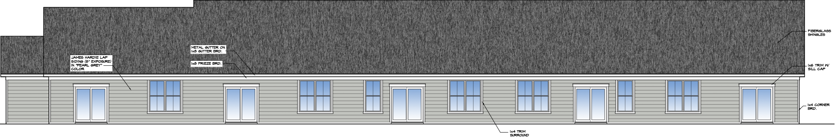
REAR ELEVATION ATTACHED 5-UNIT 3/32"=1'-0" (1/1b)
